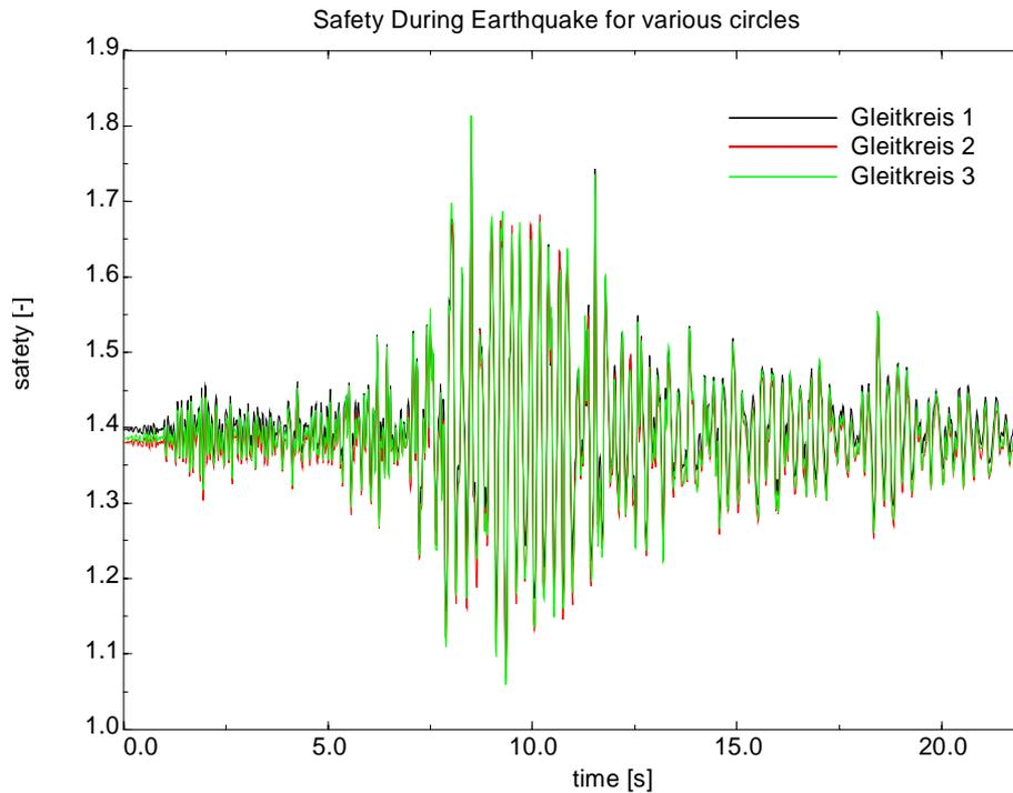
Figure 17: Time-history of safety factor for three different slope lines
