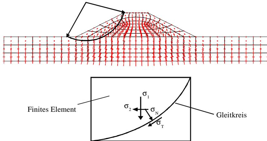
Figure 13: Circular slope and normal/tangential stress components
