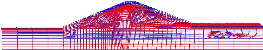
Figure 11: Displacement plot (scaling factor 100)
