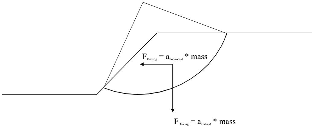
Figure 12: Krey/Bishop method for determination of slope stability
