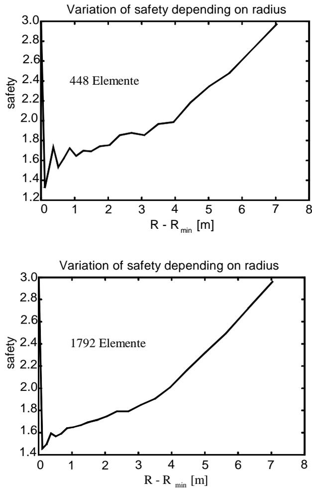
Figure 14: Safety factor for fixed central point and varying radius
