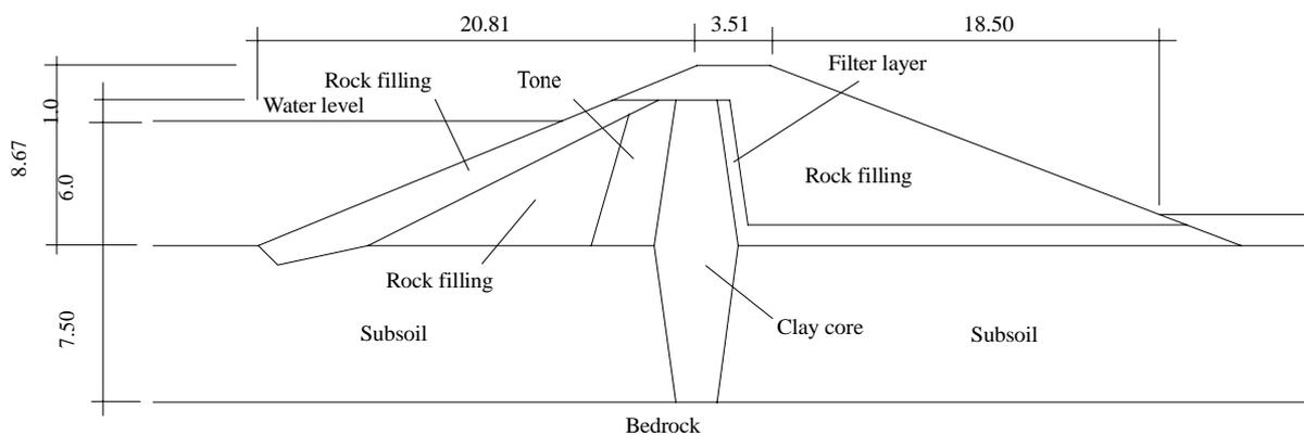
Figure 2: Dam geometry
