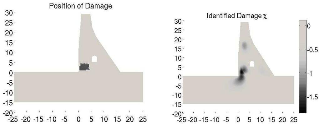
Figure 3. Left: Position of an arbitrary damage zone, Right: Reconstruction of the damage by a multifield inverse analysis. The locations of the sensors are as given in Figure 4. The Intze Wedge is not considered in the inverse analyses, since we do not expect damages there.
