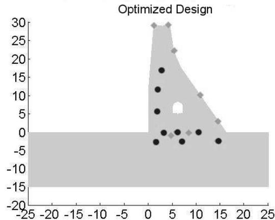
Figure 4. Optimized positions for both the pore water transducers (black points) and object points for geodetic measurements and position of extensometers (gray rhombi along downstream side and inside structure). The results have been obtained by a two field (hydro-mechanical) analysis.
