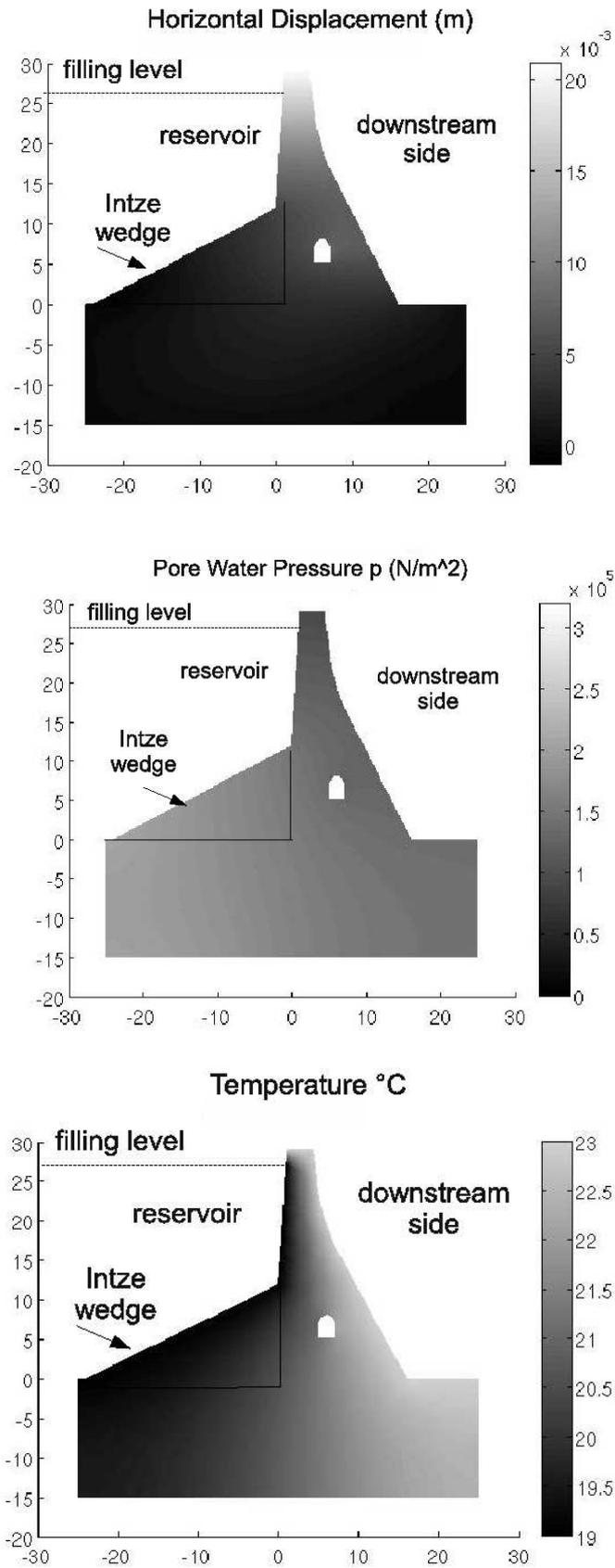
Figure 2. Simulation results: A) Deformation in horizontal direction due to hydraulic and thermal loads. B) Pore water pressure distribution in the structure. C) Thermal field for temperatures assumed to hold in September (Germany).
